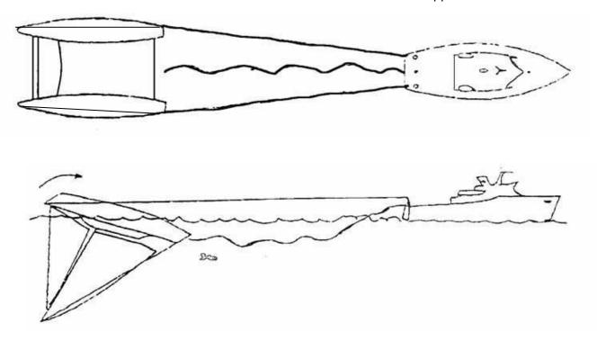
Completely ease or release central line once pull is transferred to bow lines, otherwise righting action will be prevented.
