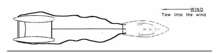
**TRIMARAN** - attach central stern line to main hull. **CATAMARAN** - attach central stern line to rear beam or short bridle from each hull.
